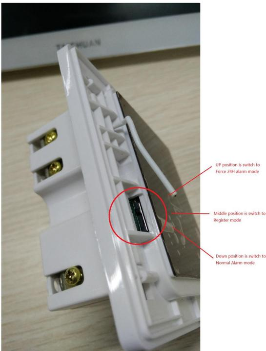
Up position is switch to 24H Force alarm mode
