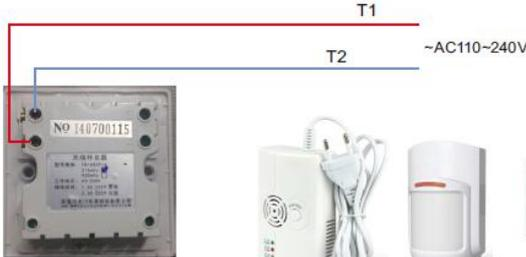
RF Signal Exchanger Wire Config
