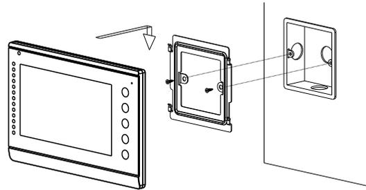
1. Embedded 86X86 embedded box on the wall, about 150cm from the ground.
