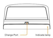
**Bracket USB Port:** Connect to the power adapter Charging for the indoor monitor.
