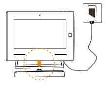
**Note:** To make sure the intercom function working continuous; When the terminal machine set on the bracket, the system will start automatically and can't be turn off manually.
