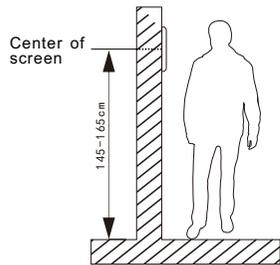
The best installation height of the indoor monitor is the center of the screen is about 145-165cm from the ground. (This data is just for reference)
