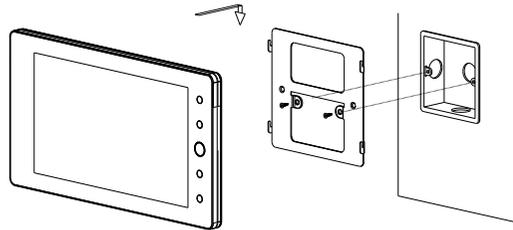
1. Embedded 86X86 embedded box on the wall, about 150cm from the ground.
